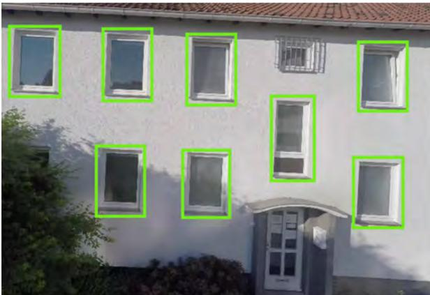
Fig. 2: Detected windows (green) in a façade image.
