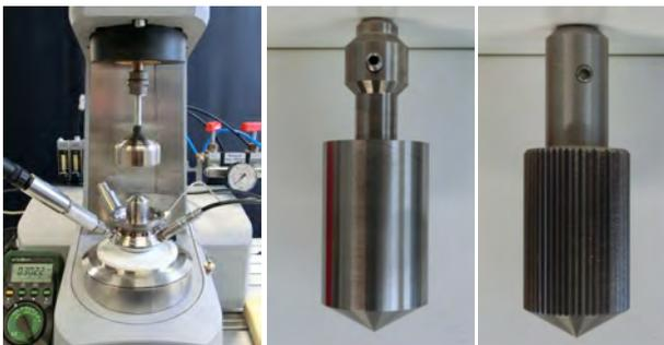
Fig. 2: Pressure cell (MC 301) (left), smooth Bob (middle) and ripped (rough) Bob (right).
