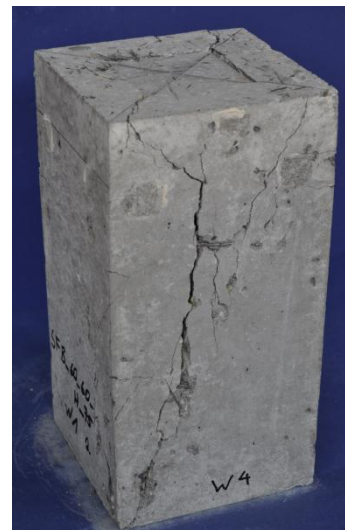
Figure 2: Specimen after partial loading test
