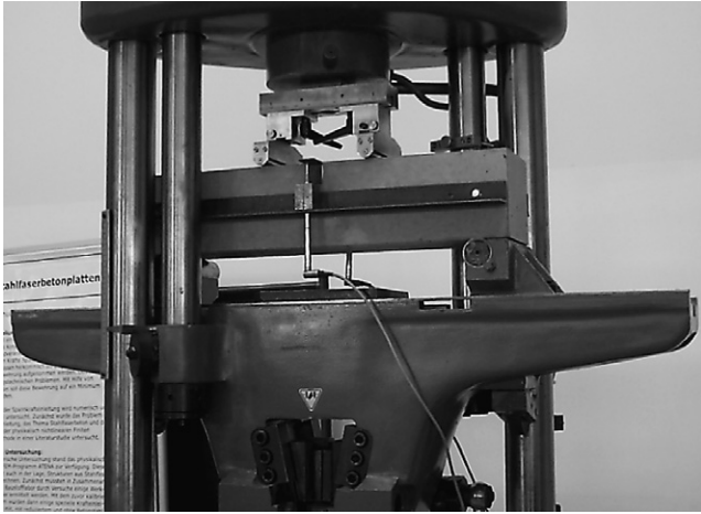
Fig. 3. 4-Point bending test to determine the flexural tensile strengths of the SFRC according to the German guideline.
