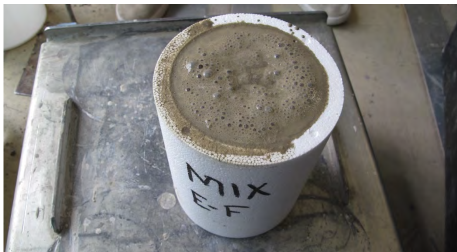
Figure 1: Compaction of a cylindrical test sample using a vibrating table
